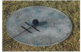
· The noise measurements were taken in accordance with IEC regulations. A windbreak net covered the microphone to minimize the effect of wind noise. The distance was
